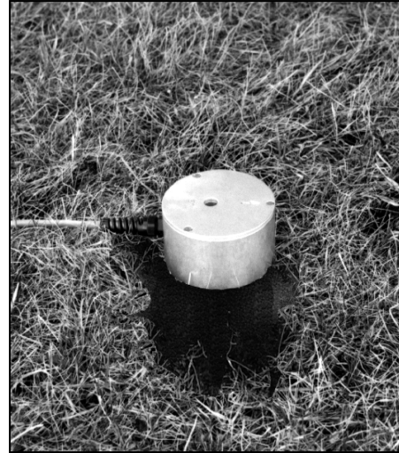
Figure 3.3 Final Installation with Ground Spikes Pushed Fully into the Ground.
