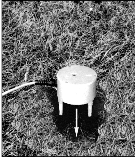
Figure 3.2 Installing the Standard Transducer using the Ground Spikes.
