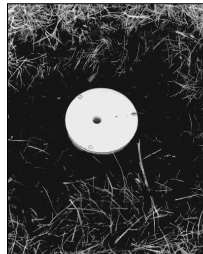
Figure 3.5 Fill In and Pack the Material around the Standard Transducer.
