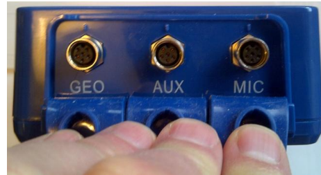
Dust Caps Pulled Back to Access Connectors
