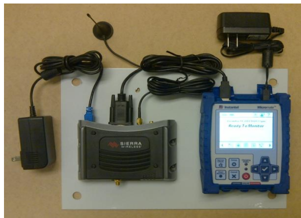
Placement of Modem, Micromate and Cables
