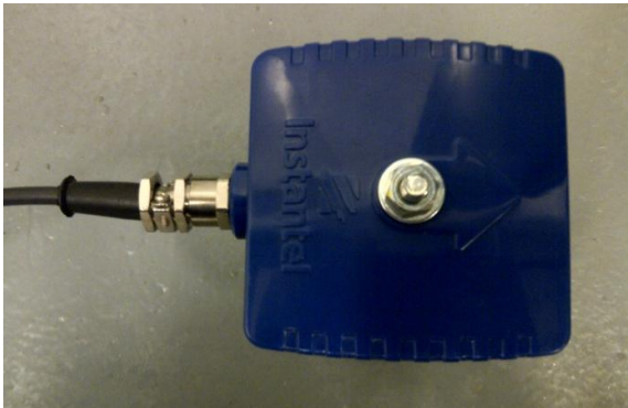
Geophone Bolted to a Floor
