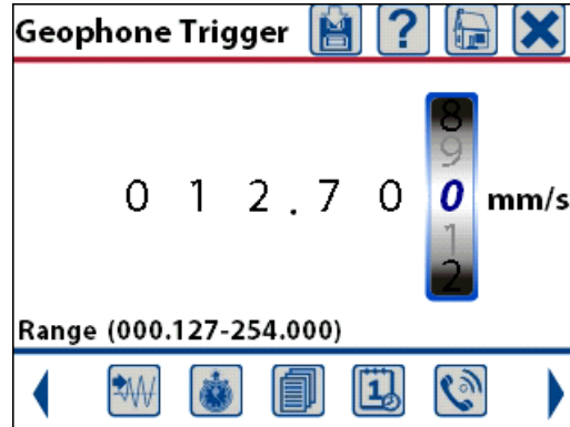
Geophone Trigger Level Set to 12.7 mm/s
