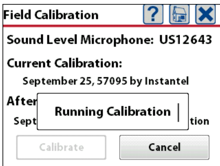
Micromate Calibrating Sound Level Microphone
