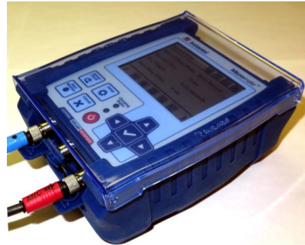
Micromate Installed in the Protective Boot
