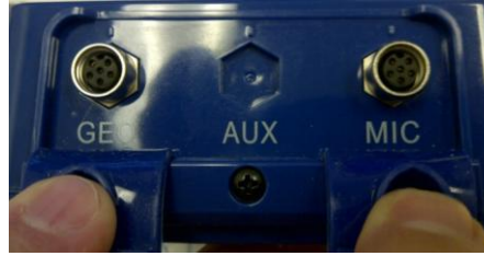
Dust Caps Pulled Back to Access Connectors
