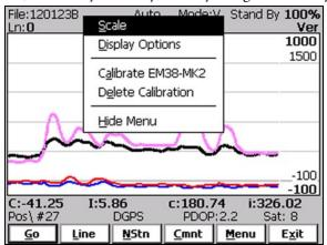
The Enter Scale dialog will be displayed. It contains four text boxes for Minimum and Maximum values of a new scale for profile plot of conductivity and Inphase. Current settings (minimum and maximum values) for the scale are displayed in the bottom right and top right corners of the plot area. Outer numbers indicate scale for conductivity and inner numbers are associated with Inphase scale. Values displayed in bold indicate the scale that is associated with grey grid lines.
