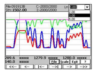
drop-down box showing the available survey lines. When the keyboard is being used you can activate the text box by pressing the **TAB** key until the drop down box is highlighted and then by using Up or Down arrow keys select one of available lines (as shown below).
