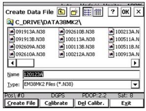
The file name can be specified in the Create Data File dialog using the Windows standard interface procedure. The EM38MK2 data files cannot be appended.
