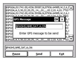
After this command is received by the GPS receiver, the confirmation message will be send by the receiver (\$PASHR, ACK\*3D) and data stream will contain the message SAT (\$PASHR, SAT,.... in the above figure).
