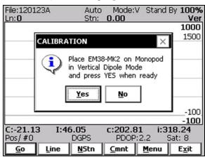
Calibration procedure is the same as described in chapter 6.1 (Monitoring Mode). Please refer to above section of the manual and follow all prompts that appear on the display. Calibration factors will be written to the data file and displayed readings will be adjusted immediately after the Calibration procedure is completed.
