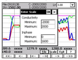
and Maximum values of a new scale for profile plot of conductivity and Inphase. Values displayed in bold indicate the scale that is associated with grey grid lines (specified earlier in Diplay Options dialog).
