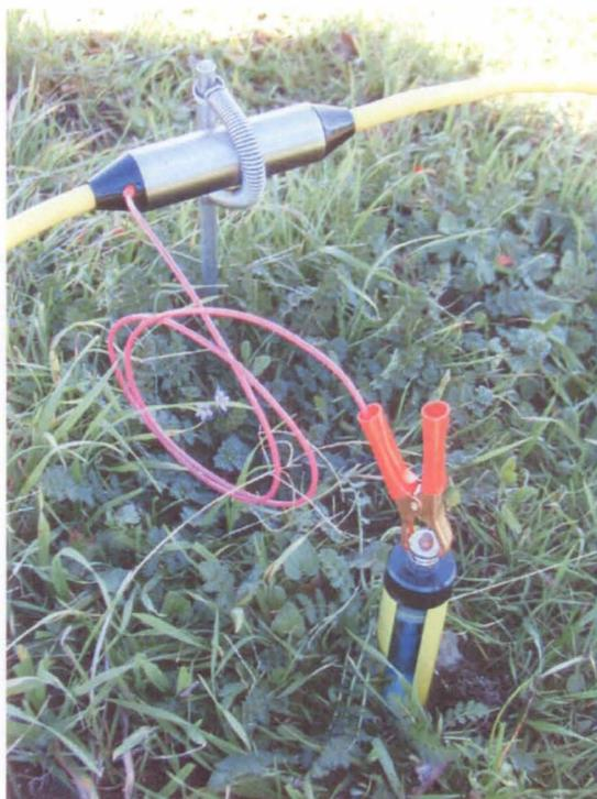
**Figure 12 Electrode in dual mode configuration.**
