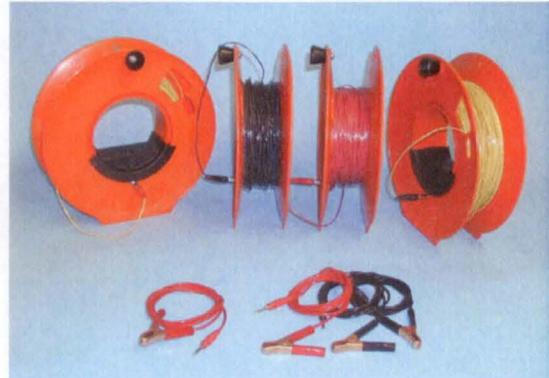
**Figure 22 Short cable set, current 2x150 m, potential 2x50m.**
