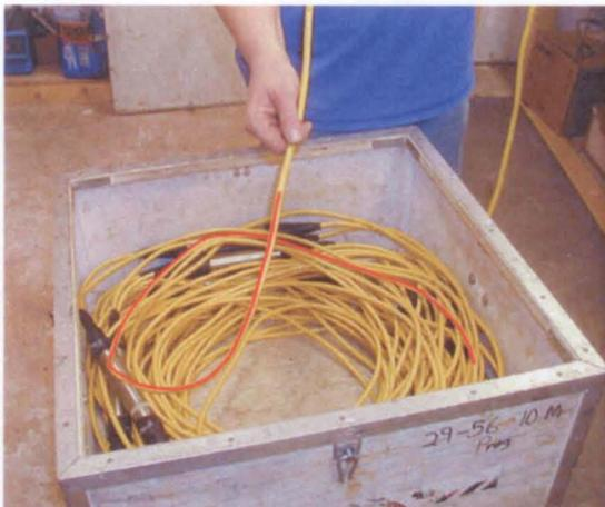
**Figure 4** Incoming cable "over" the loop.
