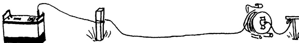
**Figure 30** Tie off cables to some fixed object to prevent cables from accidentally being pulled out of the instrument when the electrodes are moved.
