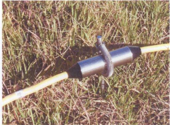
**Figure 6 Attach each switch to the stake using the stainless steel spring.**
