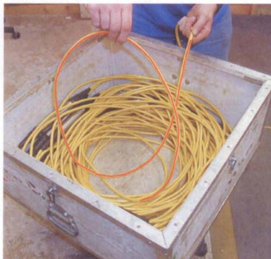
*Figure 5 Incoming cable "under" the loop.*
