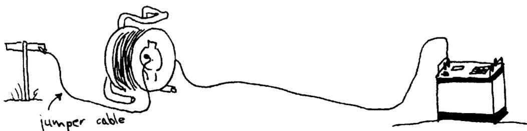
**Figure 29** Place the cable reel close to the electrode, not the instrument. Use a jumper cable to connect the reel to the electrode.
