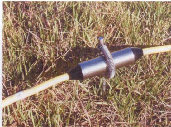
**Figure 16** Electrode used in single mode configuration.
