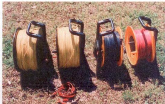
**Figure 24 Long cable set, current 2x750 m, potential 2x250 m.**
