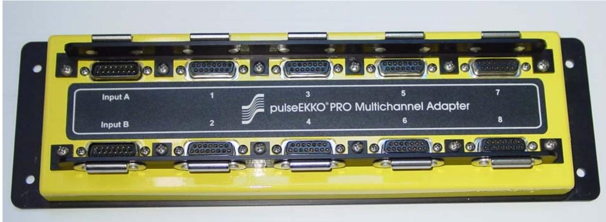
Figure J-7: Multi-Channel Adapter. The ports labelled 1 to 8 are for connecting transmitters and receivers. Inputs A and B connect to the control module.
