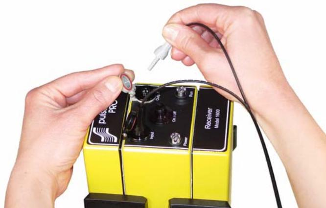
*Figure 2-13: Attaching the fibre optic cables to the transmitter and receiver. Make sure to match the connector colour to the door colour (grey to grey and black to black). Push the fibre optic cable down until you can feel it “click” into place.*
