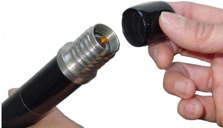
*Figure I9-4: The borehole antenna dust caps prevents the connection from getting dirty or damaged.*
