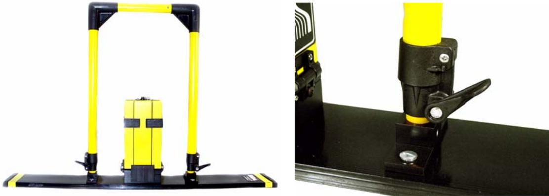
*Figure 3-2: Attach the adjustable handles to the antennas by tightening the 4 quarter-turn fasteners. Adjust the height of the handle by loosening the levers at the base of the handles (right) and pulling the handles up to the correct height.*
