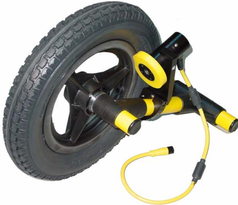
Figure 7-4: The big wheel odometer. Ensure that the small yellow odometer is tightly pressed against the rim of the wheel so that it spins when the big wheel is rotated.
