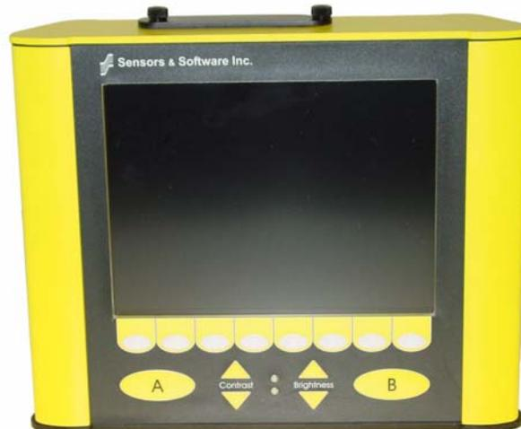
Figure 12-2: Digital Video Logger (DVL) face
