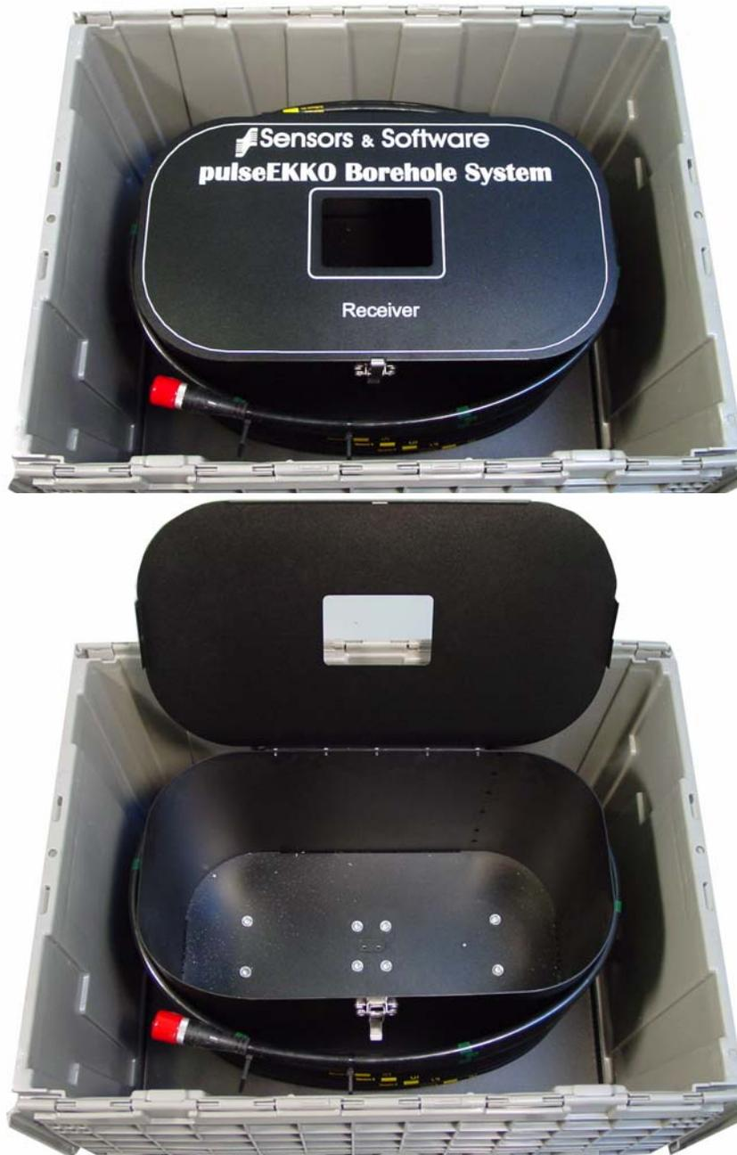
Figure I9-3: The housings for the pulseEKKO PRO receiver and transmitter electronics are mounted inside the grey shipping cases.
