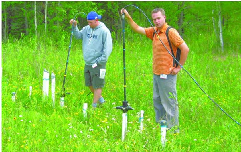
Figure 16-20: Cross hole transillumination surveys with the pulseEKKO PRO system require the use of 50, 100 or 200 MHz borehole antennas available from Sensors & Software. See Appendix I: pulseEKKO PRO Borehole Data Acquisition for more details.
