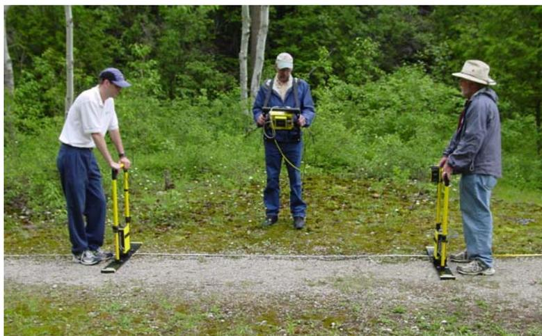
*Figure 16-17: CMP field operation.*
