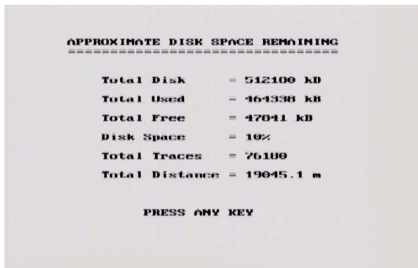
Figure 18-5: View Disk Space screen. The total amount of disk space remaining is expressed in kilobytes, a percentage of the total disk space, number of traces and total distance. The last two values are calculated using the current setup parameters.
