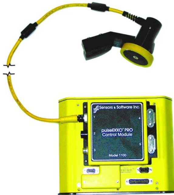
*Figure 11-6: The pulseEKKO PRO accepts input from various odometers including the wheel odometer shown, which is from the SmartCart. Odometers attach to receptacle 1 on the control module or to the transducer end of the transducer cables. When using the Big Wheel Odometer with low frequency antennas, use a long extension cable (not shown) to attach to receptacle 1 on the control module*
