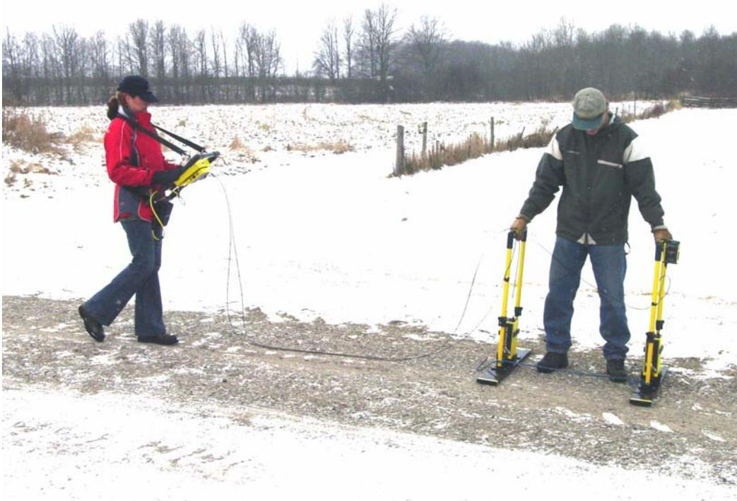
*Figure 16-1: Two person data collection with the pulseEKKO PRO system. The antenna operator moves the antennas to each data location point. The data trace is collected by the DVL operator using the electrical beeper/trigger or the DVL button. The data trace can also be collected by the antenna operator using the fibre optic beeper/trigger. The data are visible in real time on the DVL screen.*
