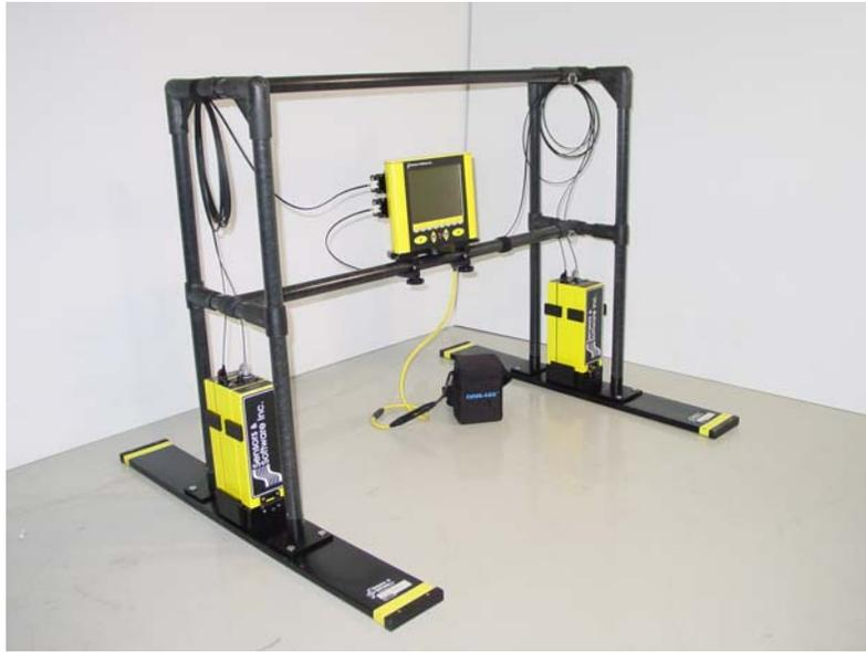
*Figure 4-2: Complete One-Man Handle Assembly. The DVL tray can be attached to the middle bar (as shown), the top bar or the DVL can be carried by a second operator. In the configuration shown, the DVL can be a source of noise so, if you see banding in the data, this may be alleviated by moving the DVL away from the receiver.*
