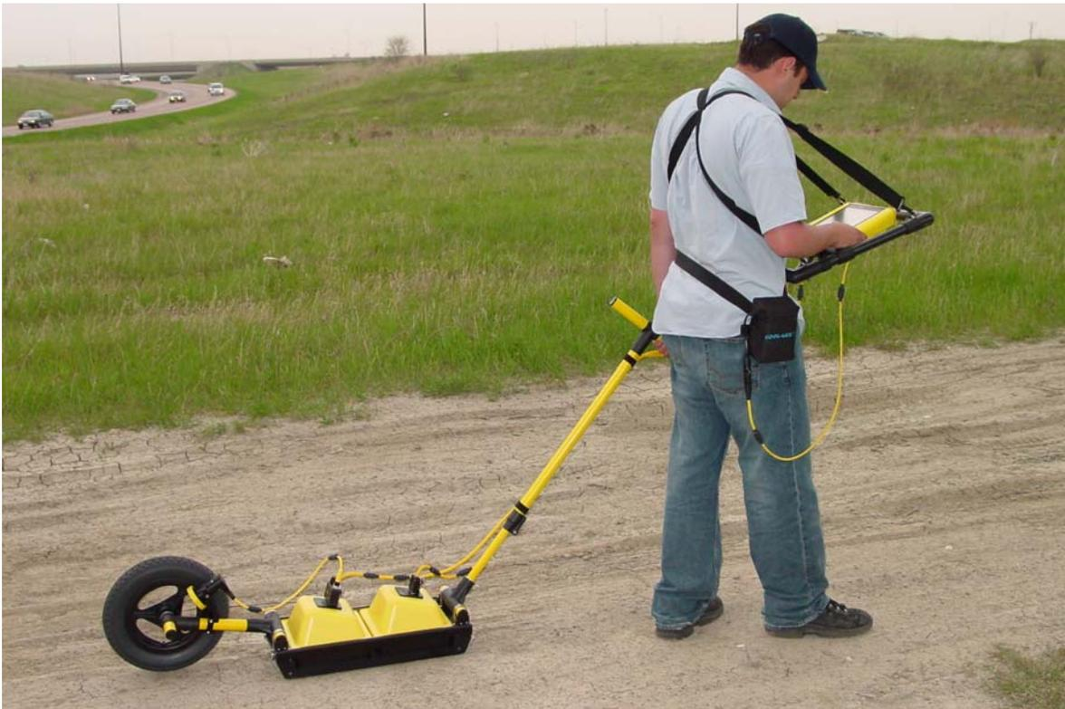
*Figure 16-8: Hand Tow operation. As the operator drags the transducers across the surface, the odometer triggers data collection at equally-spaced intervals (called the Step Size). The data being collected are visible in real time on the DVL screen.*
