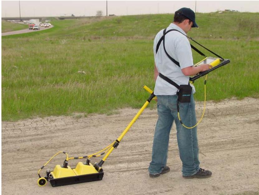
*Figure 16-9: Hand Tow mode using Small Wheel Odometer.*
