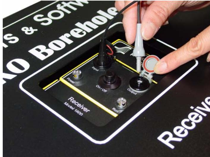
Figure I9-12: Attaching the fibre optic cables to the transmitter and receiver. Make sure to match the connector colour to the door colour (grey to grey and black to black). Push the fibre optic cable down until you can feel it “click” into place
