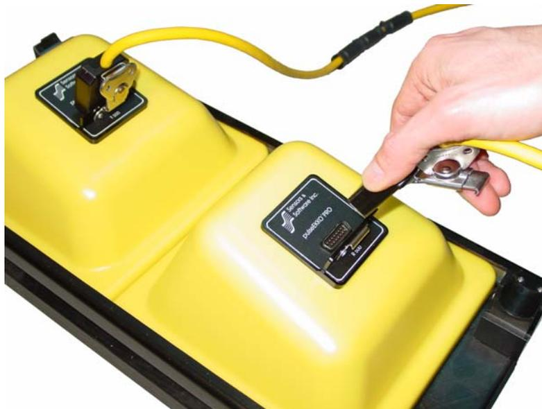
*Figure 2-18: Connecting the transducer cables to the transducers. The connections are secured with latches.*
