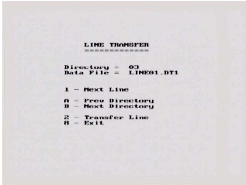
*Figure H-1: Line Transfer screen. Use the A and B button to select one of the 20 available directories, then use the 1 button (Next Line) to move through the data lines in the directory. When the name of the data line to transfer appears, press 2 (Transfer Line) to send it to the PC.*
