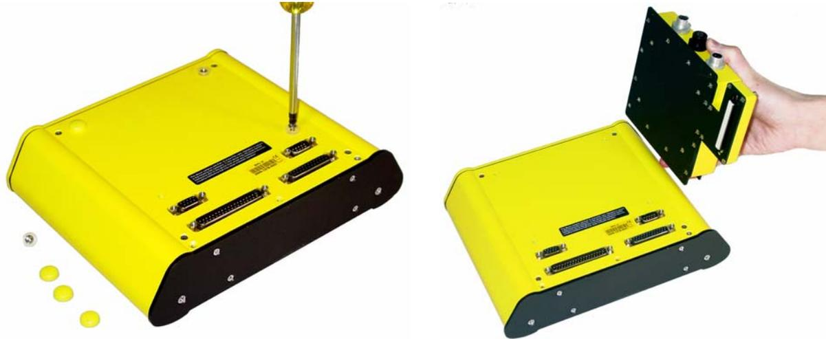
Figure 2-2: Remove the 4 yellow caps and the 4 screws from the back of the DVL (left) and place the control module on the back of the DVL (right). Make sure that the 37 pin connector is aligned properly with the 37 socket connector on the control module.
