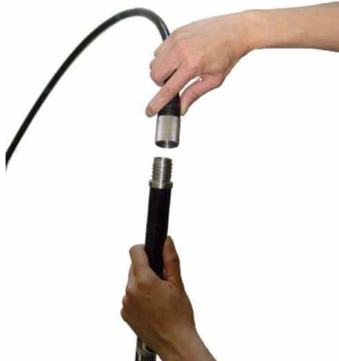
*Figure I9-10: Connect the borehole antenna to the borehole cable by twisting into place. Ensure a snug connection to prevent water from leaking in.*
