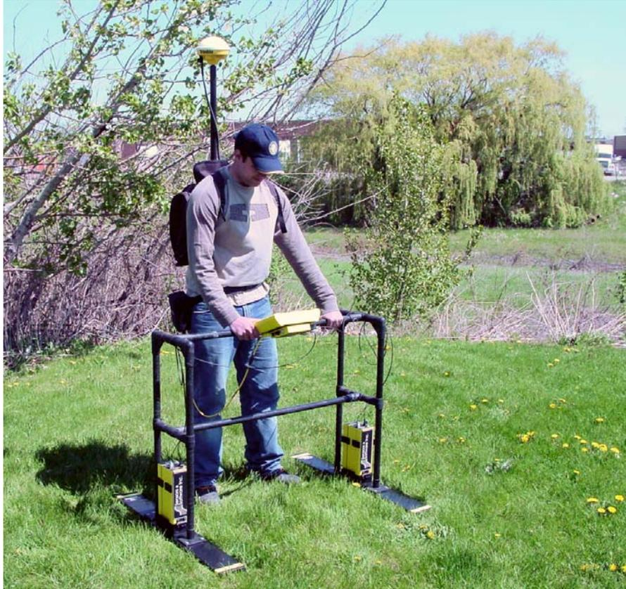
*Figure 16-5: One man handle setup. The operator moves the antennas to each data location point and collects the trace using the DVL B button. The data are visible in real time on the DVL screen.*
