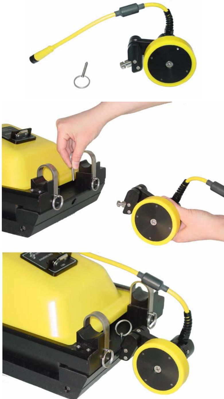
*Figure 7-6: The small wheel odometer (top) attaches to the skid plate assembly by inserting the metal post into the hole on the end of the skid plate (middle). The odometer is secured into place by inserting the metal pin into the vertical hole on the edge of the skid plate (bottom).*
