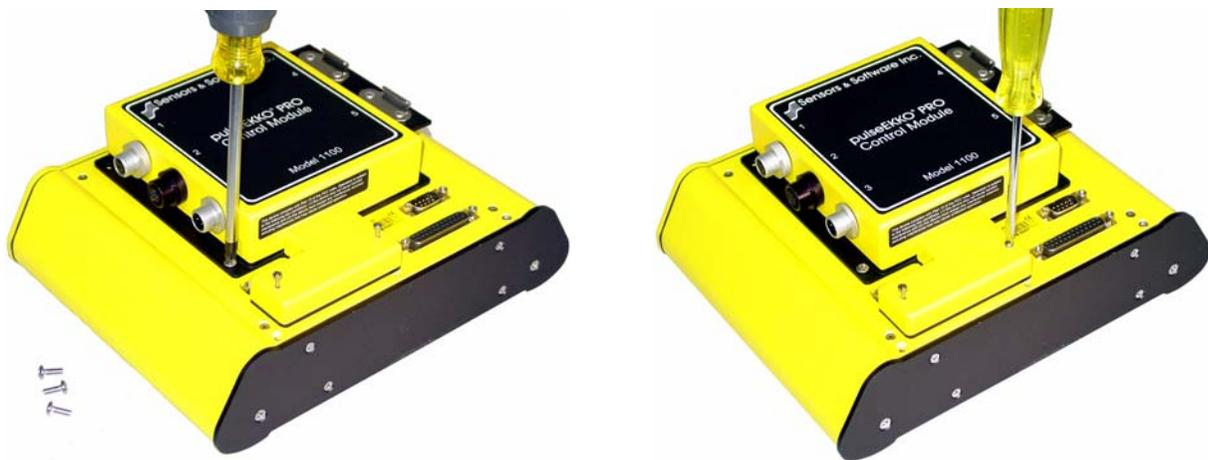
Figure 2-3: Attach the control module to the DVL using the 4 screws supplied (left) and a Phillips screwdriver (not supplied). Tighten the 37 pin connectors into place (right) with a small slotted screwdriver (not supplied).
