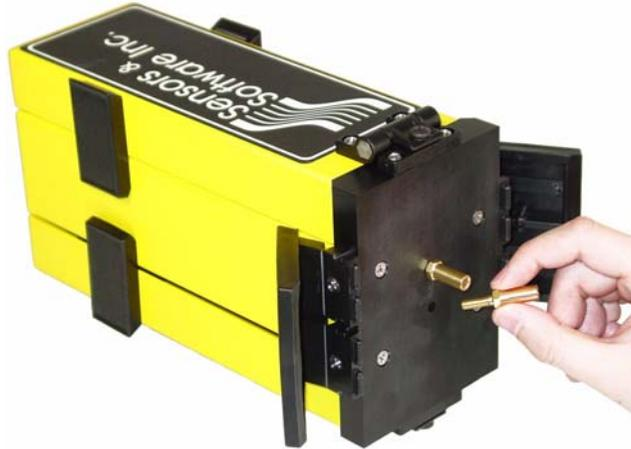
*Figure 2-6: Hand tighten the brass sockets into the bottom of the transmitter and receiver.*
