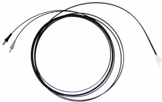
*Figure 2-12: Dual fibre optic cable used with the transmitter and receiver. The black and grey strain reliefs on the end of the cable (left) plug into the same coloured fibre optic receptacles on the top of the transmitter and receiver (see Figure 2-13). The connection on the other end of the cable (right) connects to either fibre optic receptacle on the control module (see Figure 2-14).*
