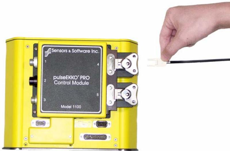
*Figure 2-14: The dual fibre optic cable from the transmitter and receiver attaches to the electrical to fibre optic converters on the control module. The fibre optic cable from the transmitter connects to the control module receptacle labelled 4 while the fibre optic cable from the receiver connects to the control module receptacle labelled 5. This connection is keyed so it will only attach when the fibre optic cable is in the orientation shown.*
