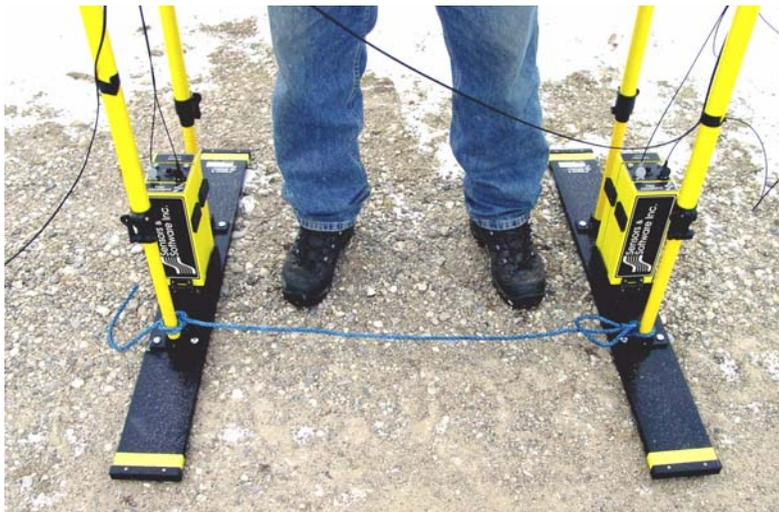
*Figure 16-4: When using the adjustable handles, the antenna separation can be maintained by using a length of rope tied between the antennas.*
