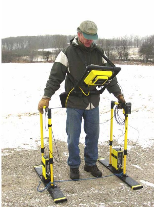
*Figure 16-2: One person operation setup. The operator moves the antennas to each data location point and collects the trace using the fibre optic beeper trigger. The data are visible in real time on the DVL screen.*
