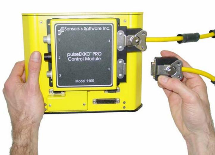
*Figure 2-19: Connecting the transducer cables to the Control Module. The transducer cables from the transmitting and receiving transducers connect to the control module into either the receptacle labelled 4 or 5. The “smart” electronics figures which device is connected to which receptacle. The cable attachments are secured with latches.*
