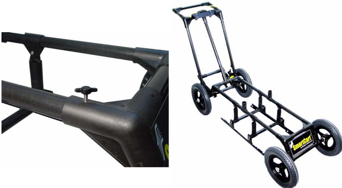
Figure 5-3: Attach the separation bars to the front and rear axle assemblies of the SmartCart using the finger screws (left). Be careful to align the screws so they go in straight. If the screws are forced in the threads can be stripped. The SmartCart with the 0.5m separation bars attached is shown on the right.
