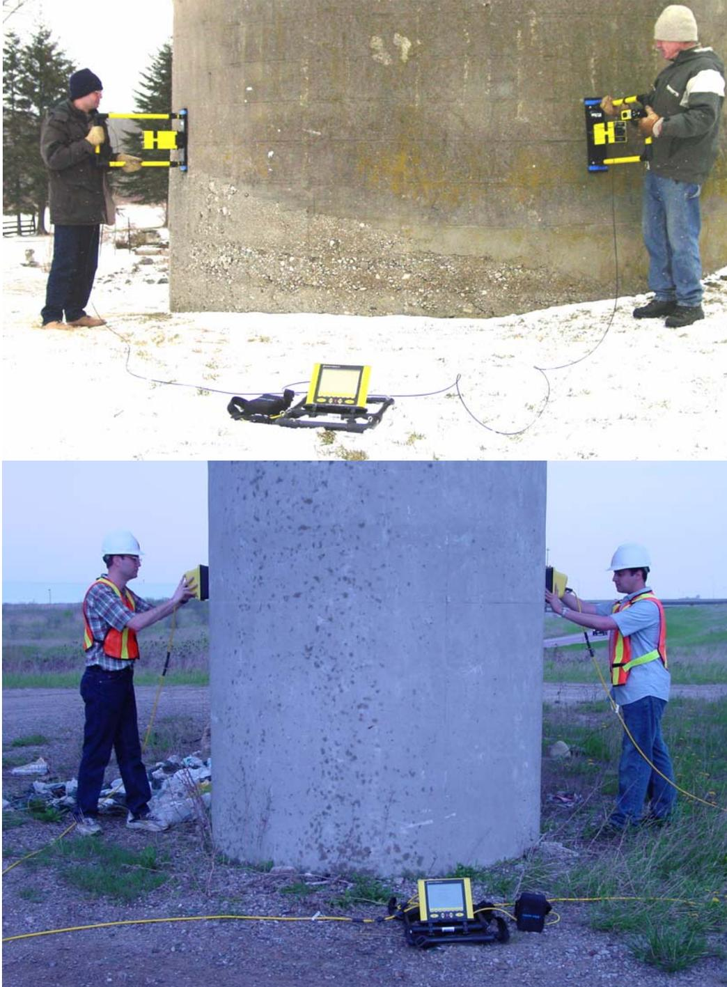
*Figure 16-21: Transillumination survey setup with antennas (top) and transducers (bottom). With a transillumination survey, the GPR signal is sent from the transmitter directly to the receiver after it has passed through a structure. The DVL is centrally located and data acquisition is controlled by either triggering the system with the electrical or fibre optic beeper/trigger or using Free Run mode with a time delay between traces.*
