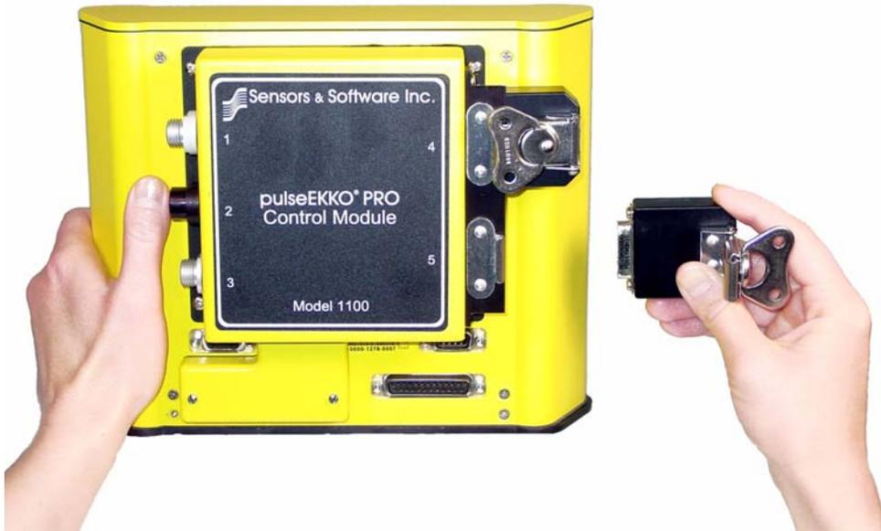
*Figure 2-4: Low frequency antennas (12.5 to 200 MHz) require the electrical to fibre optic converters to be attached to the control module and secured using the latches.*
