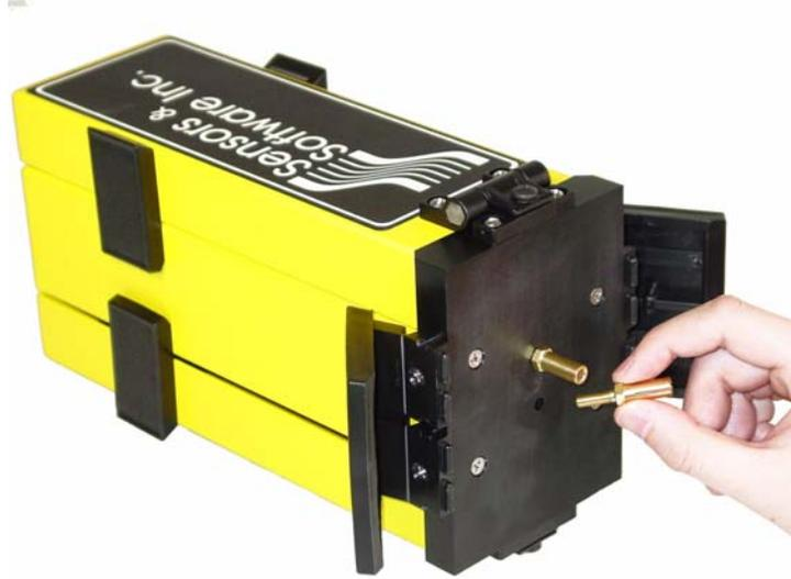
*Figure I9-6: Hand tighten the brass sockets into the bottom of the transmitter and receiver.*
