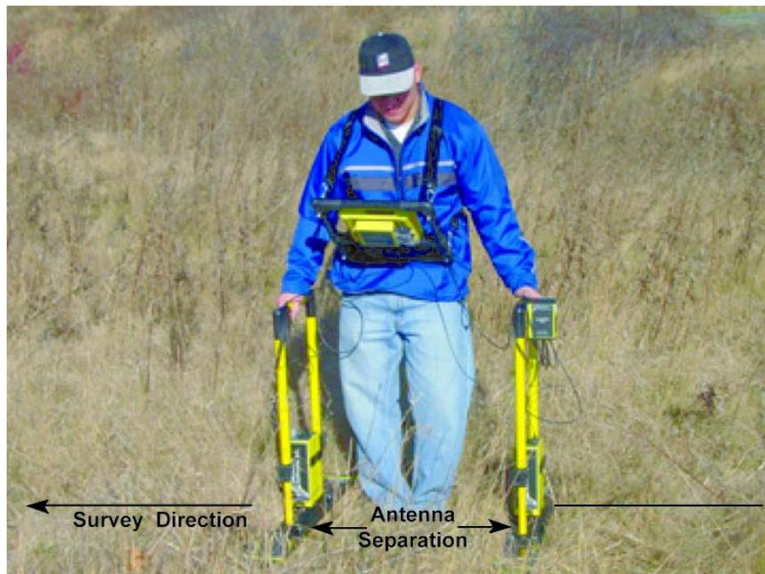
Figure 16-13: Most common reflection surveying technique. Antennas are held at the proper antenna separation for the selected frequency and perpendicular to the survey line direction. This antenna orientation ensures the maximum in-line GPR energy and reduces reflections from off-line targets.
