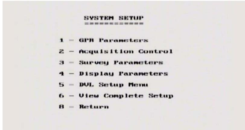
Figure 13-1: The System Setup main menu is used to access and change any parameter used for data collection. Related parameters are grouped under different menu headings, for example, GPR Parameters list the variables specific to the GPR system. Select View Complete Setup from this menu to quickly locate the desired parameter and the heading it is listed under.
