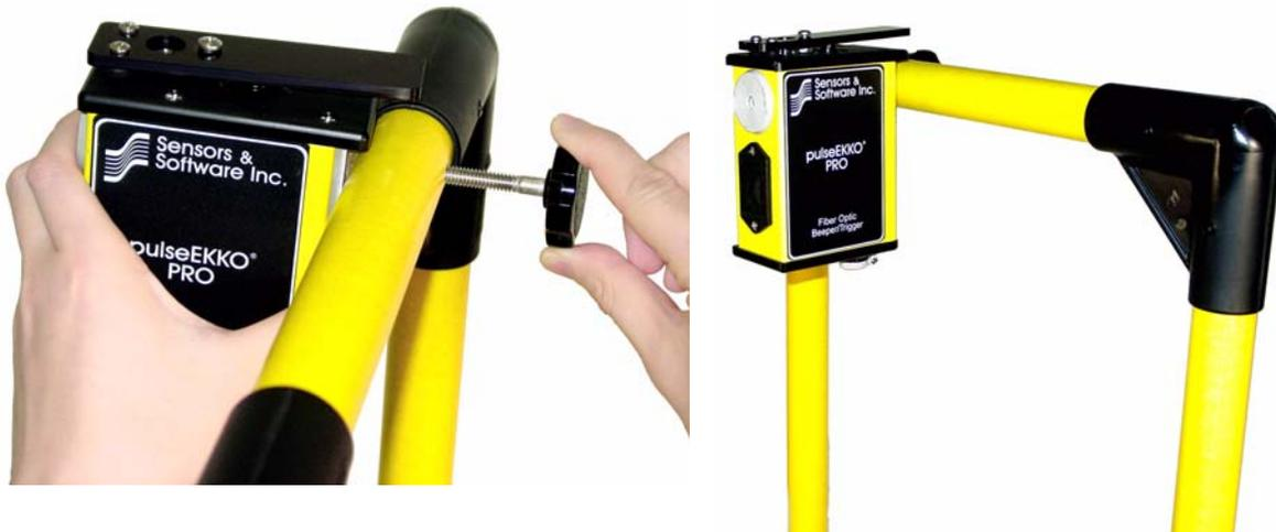
Figure 11-2: Attaching the Fibre Optic Remote Beeper/Trigger unit to the transmitter handle.
