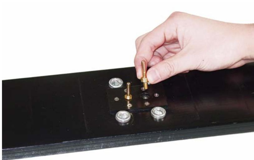
*Figure 2-7: Insert the male brass antenna pins into the holes on the top of the antenna and finger-tighten.*
