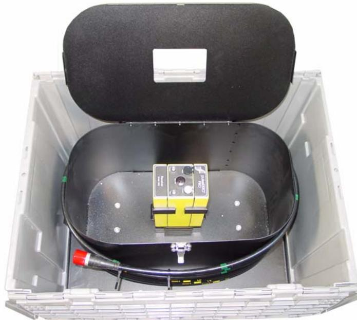
*Figure I9-7: Attach the transmitter and receiver to the mounting blocks in the bottom of the housings and secure into place using the latches. For consistent signal polarity, ensure the transmitter and receiver are oriented the same way with respect to one another.*
