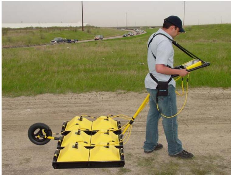
*Figure J-1: Fixed frequency 2D array multi-channel data collection.*
