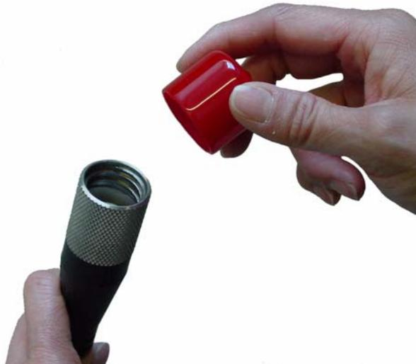
Figure I9-9: Remove the dust cap from the end of the borehole cable. When storing the borehole housings always use the dust cap to protect the connector.
