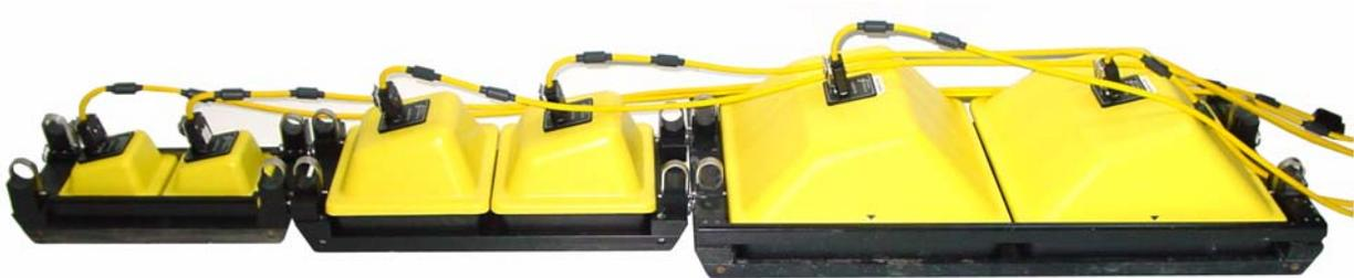
Figure J-3: Multiple-frequency, in-line mode of multi-channel data collection.
