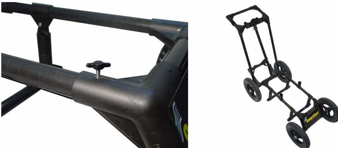
Figure 8-2: Attach the separation bars to the front and rear axle assemblies of the SmartCart using the finger screws (left). Be careful to align the screws so they go in straight. If the screws are forced in the threads can be stripped. The SmartCart with the 500 MHz separation bars attached is shown on the right.
