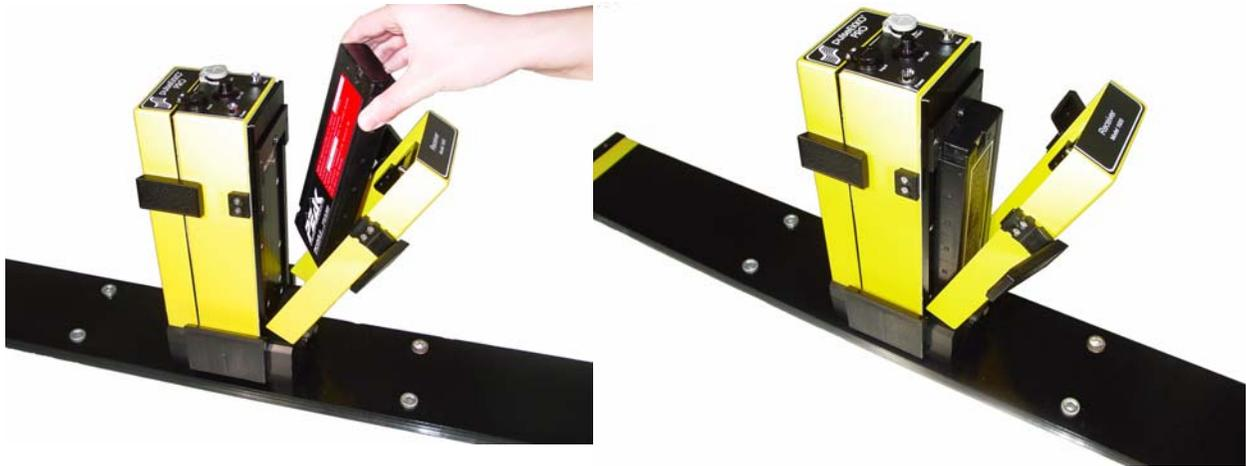
Figure 2-11: Insert the 12 Volt battery into the battery compartment making sure that battery polarity is correct. The positive (+) terminal faces inward. The battery is “keyed” so it will only seat properly in the compartment if it is in the correct orientation.
