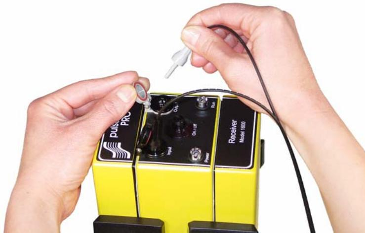
Figure 17-2: Make sure fibre optic strain relief colour matches the receptacle door colour (grey to grey and black to black).
