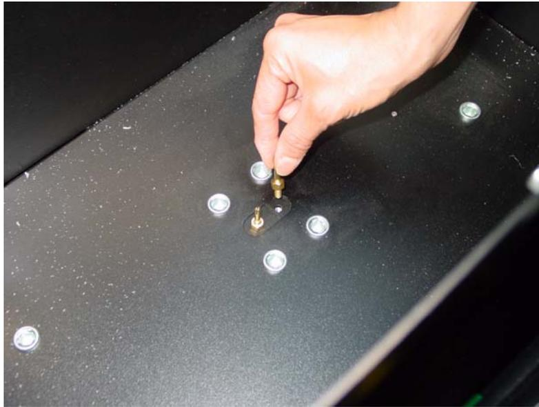
Figure I9-4: Insert and hand tighten the two male brass antenna pins into the bottom of the housing (bottom).
