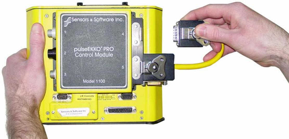
Figure 9-4: Connecting the TR1000 Adapter cable to the Control Module. The end with the extra receptacle on the side needs to be attached to the bottom receptacle on the Control Module.
