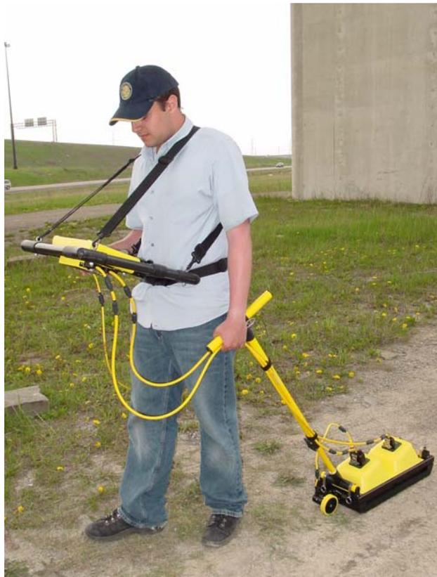
*Figure 16-10: The Small Wheel Odometer can be put on either end of the transducer skid plate.*
