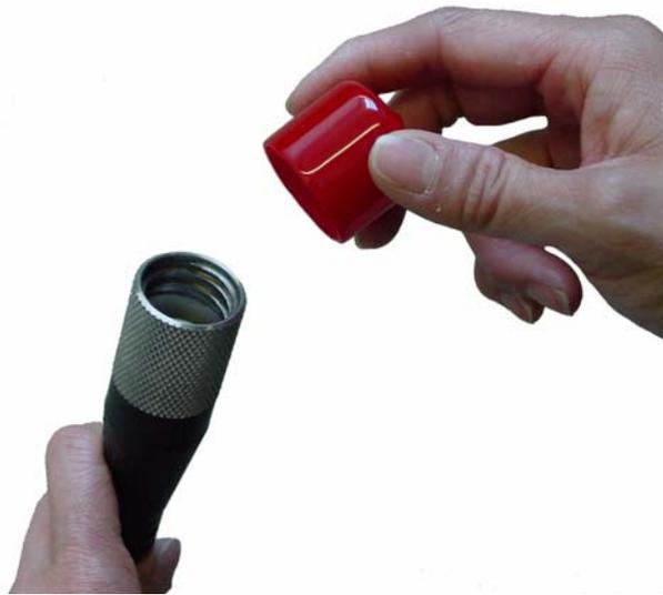
*Figure I9-3: The borehole cable dust caps prevents the connection from getting dirty or damaged.*
