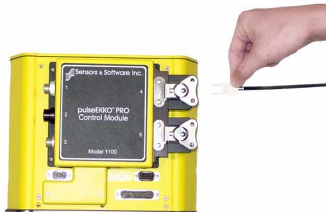
Figure I9-13: The dual fibre optic cable from the transmitter and receiver attaches to the electrical to fibre optic converters on the control module. The fibre optic cable from the transmitter connects to the control module receptacle labelled 4 while the fibre optic cable from the receiver connects to the control module receptacle labelled 5. This connection is keyed so it will only attach when the fibre optic cable is in the orientation shown.
