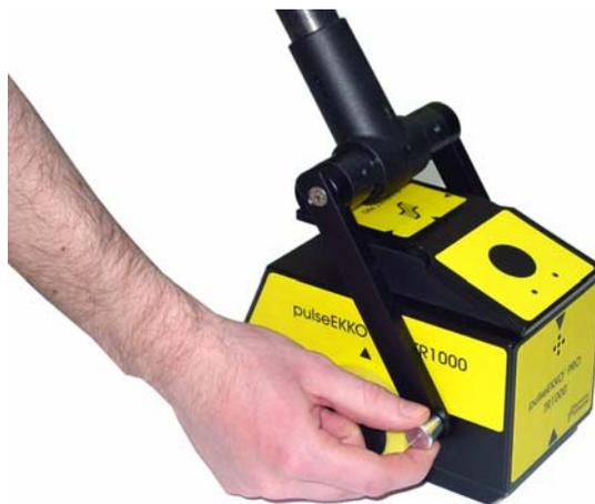
*Figure 9-9: Attach the handle to the front mounting holes when scanning vertical walls or for situations when it is preferable to collect data by pulling the TR1000 towards the operator.*
