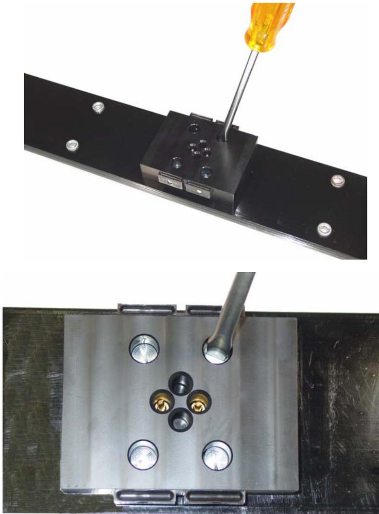
*Figure 2-8: Attach the mounting blocks to the top of the antenna using the 4 quarter-turn fasteners. Before doing so, make sure that the 2 male brass antenna pins have been screwed into the top of the antenna first.*
