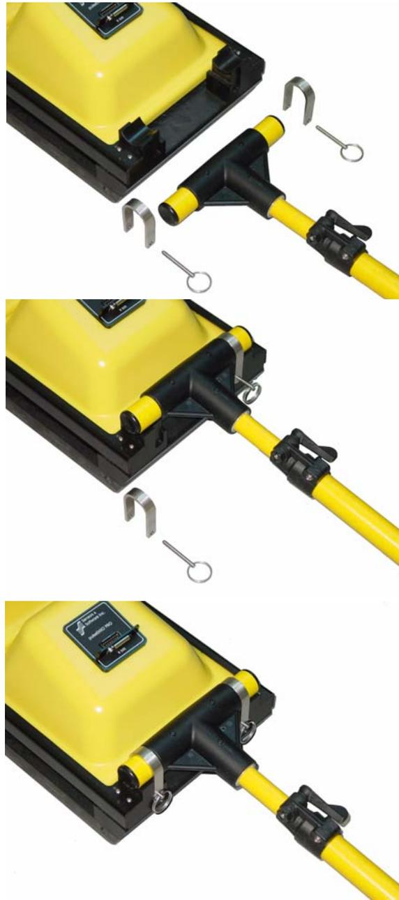
*Figure 7-2: To attach the adjustable tow handle to the skid plate assembly, place the T end of the handle into the trough on the end of the skid plate assembly where the receiving transducer label is facing. The T end of the handle is attached to the skid plate assembly by placing the U-bracket over the top and into the vertical slots. The handle is secured into place by inserting the metal pins into the holes at the bottom of the U bracket.*
