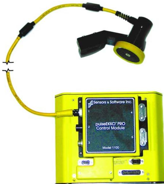
Figure 5-7: The SmartCart odometer connects to receptacle 1 on the control module.
