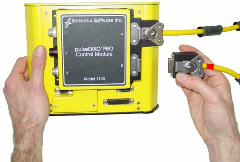
Figure J-9: A standard transducer cable is connected and latched to the top receptacle (#4) on the control module. The Multi-Channel Adapter Cable is connected and latched to the bottom receptacle (#5) on the control module.
