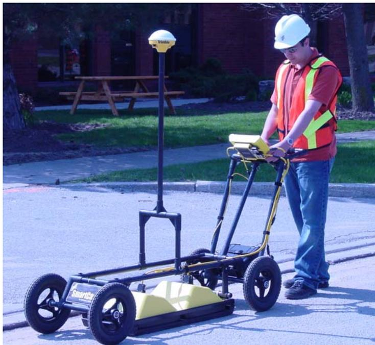
*Figure 16-11: The SmartCart has separation bars to accommodate the 250, 500 and 1000 MHz transducers.*
