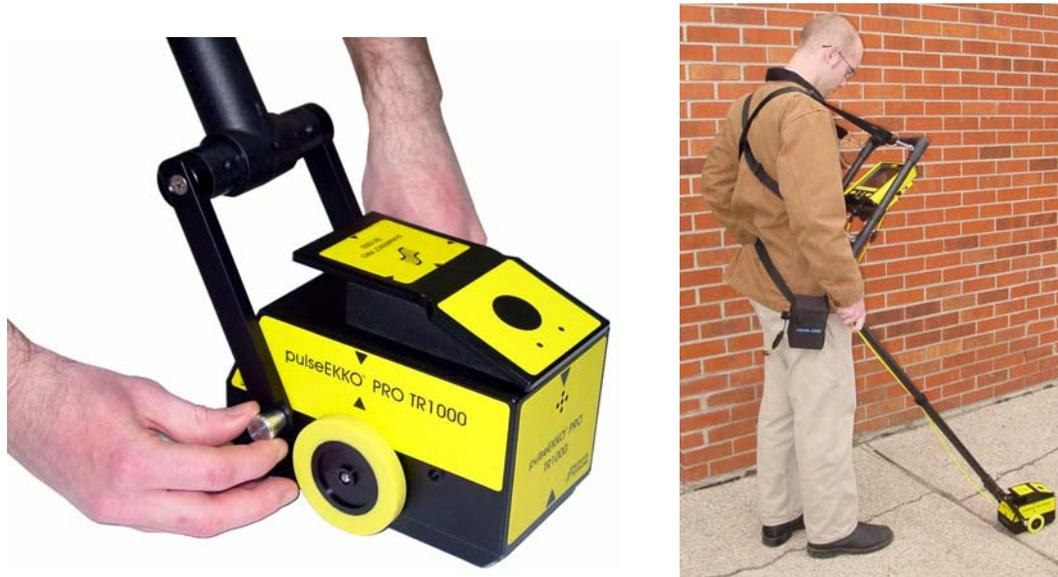
*Figure 9-8: Attaching the handle to the rear mounting holes (left) allows the TR1000 to be deployed from a standing position (right).*
