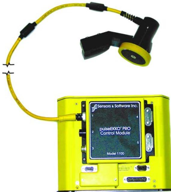
Figure 8-6: The SmartCart odometer connects to receptacle 1 on the control module.
