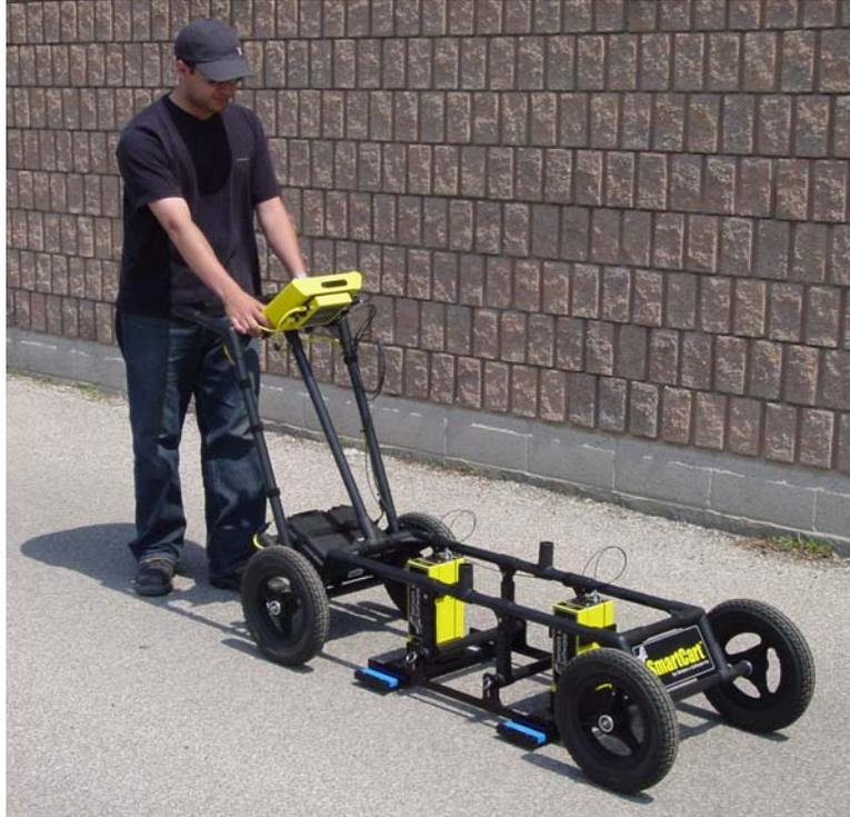
Figure 16-6: The SmartCart has 0.5m and 1.0m separation bars to accommodate the 50, 100 and 200 MHz antennas.
