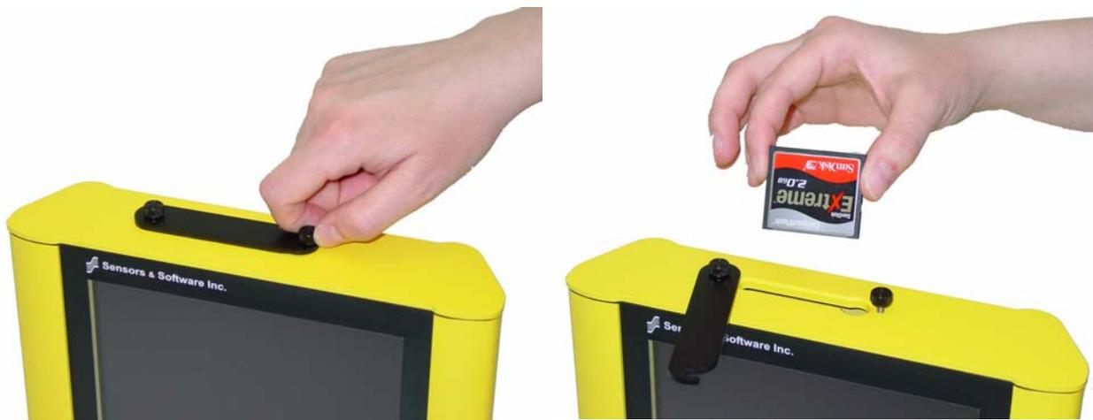
Figure: 12-3 The DVL has a removable compact flash drive for data storage.
