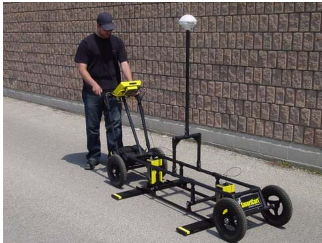
Figure 16-15: Various system configurations with GPS added. Ideally, the GPS should be positioned near the mid-point of the GPR antennas.
